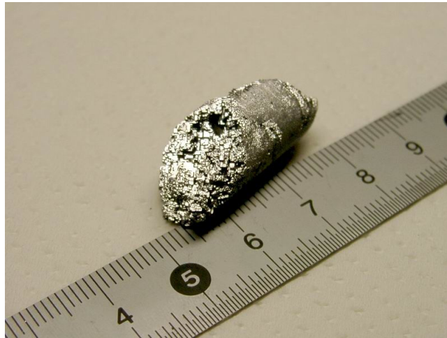
Figure 1. Image of a typical single crystal grown using the Sb-flux method. (This figure is in colour only in the electronic version)
